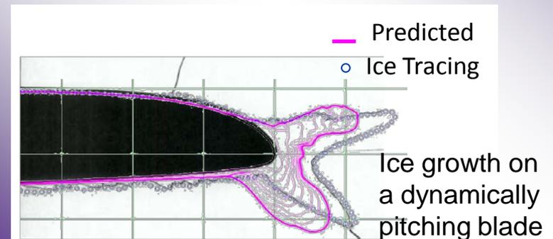
**NRTC/VLC Project: High Fidelity Icing Analysis and Validation for Rotors (WBS No. 2012-B-11-T1.1-P2)**
