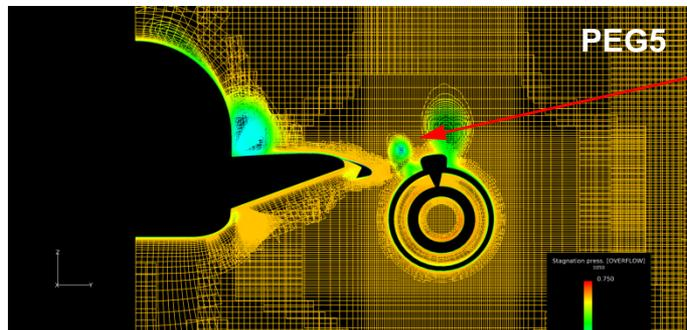
Not enough grid resolution to adequately resolve the chine vortex as it convects up and over the main wing
