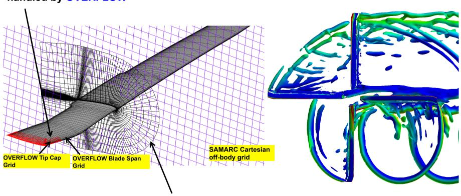
Outer boundary overset communication b/w near-body OVERFLOW grid and off-body SAMARC grid handled by PUNDIT
