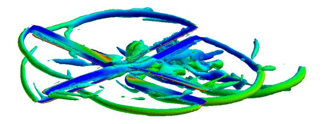
Iso-surfaces of Q criterion computed on-the-fly using the ParaView plug-in
